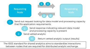
Purpose: Compute nodes serving critical infrastructure operate at different, potentially austere locations. In this environment, the exchange of information between analytic producing and consuming nodes depends on common frameworks to support interactions among nodes.
